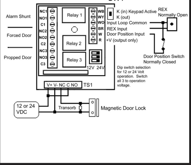
Basic Access Control with an Electric Door Strike
